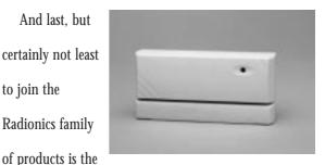
DS1109i Glass Break Detector. It uses microprocessorbased Sound Analysis Technology (SAT) to listen for the specific frequencies associated with breaking glass. It can be used to detect breakage of Plate, Tempered, Laminated and Wired glass types. A built-in environment test feature alerts the installer of false alarm hazards in harsh environments. It is specially designed to be mounted on door and window frames. A built-in magnetic contact allows monitoring of a door or window opening.
